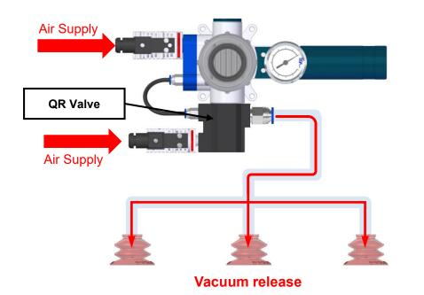
✓ When vacuum is released, release air is passing through the release control valve with QR-valve to release vacuum.
