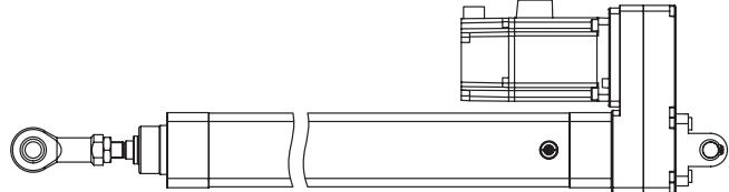
Using the diagram of the maximum axial loading as a function of the absolute stroke, the maximum axial load depending on the given mounting case can be obtained as  $F_{\text{max}} = 700 \text{ N}$ .
