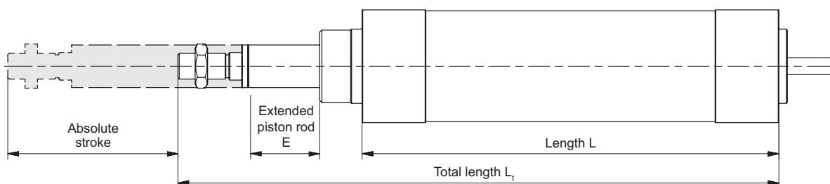
**Absolute stroke = Effective stroke + 2 × Safety stroke**
