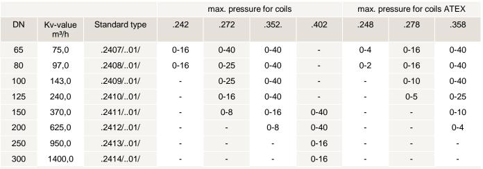
The flow rate mentioned in the table applies to the strongest coil. Max. pressure 16 bar with EN-GJL-250 body PN16
